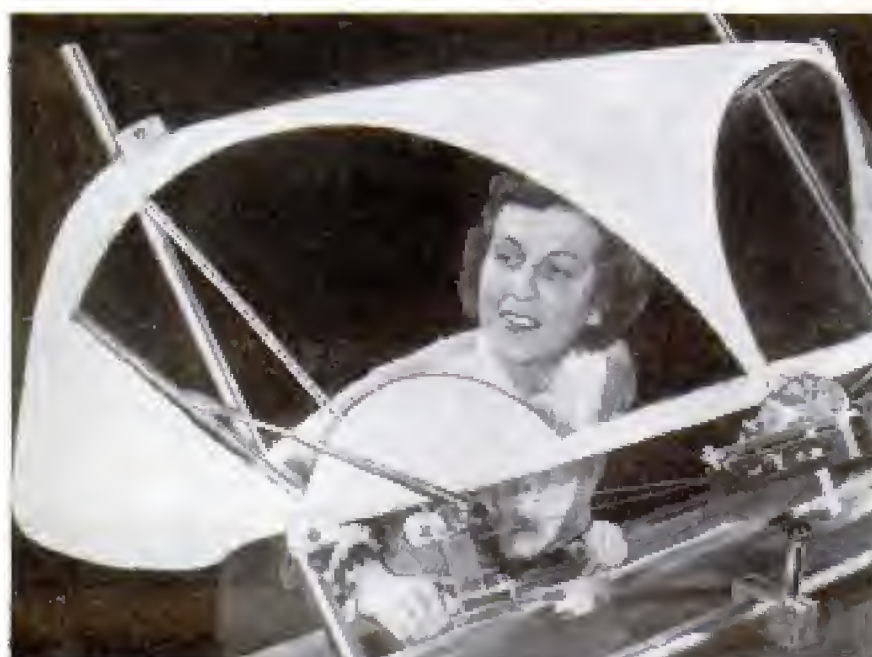
Dotted line is where usual blade stops. New type wiper wiper 5½ inches more
